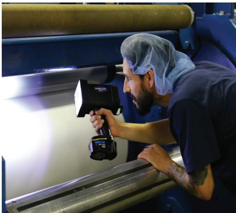
The handheld Unilux H2 Series LED strobe can be used to inspect any location on the running process line for defects like skips or voids that can be caused by plugged holes in
