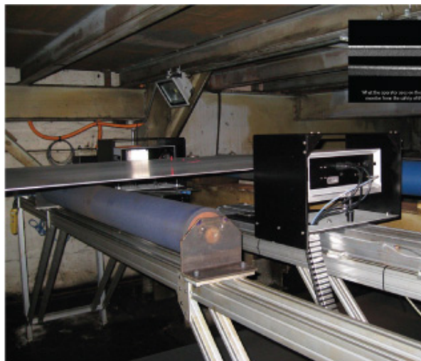
Edge Tech's on-screen view of 100% of the knife circumference (inset) enable operators to make adjustments to maintain specifications and schedule knife maintenance before conditions lead to defects.
